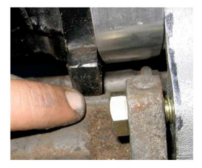
IT MAY BE NESSECARY TO GRIND A SMALL AMOUNT OFF OF THE BLOCK TO ALLOW THE STARTER TO BOLT FLUSH TO THE TRANSMISSION. TORQUE STARTER BOLTS TO PROPER VALUE.
