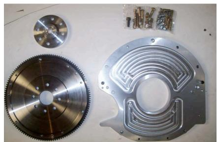
YOUR WILCAP FLYWHEEL IS DRILLED FOR THE 10 1/2" (10.4) CLUTCH COVER (PRESSURE PLATE) PATTERN. CONTACT WILCAP FOR SPECIFIC PRESSURE PLATE AND CLUTCH APPLICATIONS.
