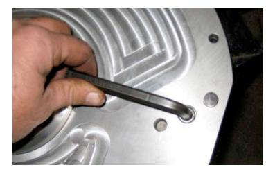
INSTALL THE CAP SCREW AND THE SOCKET HEAD CAP SCREW WITH THREAD LOCKING COMPOUND AND TORQUE, CHECK TO MAKE CERTAIN THAT THE BOLTS DO NOT PROTRUDE FROM THE SURFACE OF THE ADAPTER PLATE. IF NEEDED, TRIM THE BOLT HEAD OR SHANKS SO THAT IT IS FLUSH OR BELOW THE SURFACE OF THE ADAPTER PLATE.
